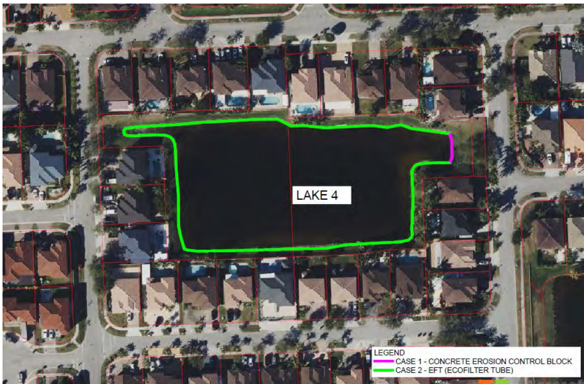
Figure 23: Aerial of recommended erosion control elements
