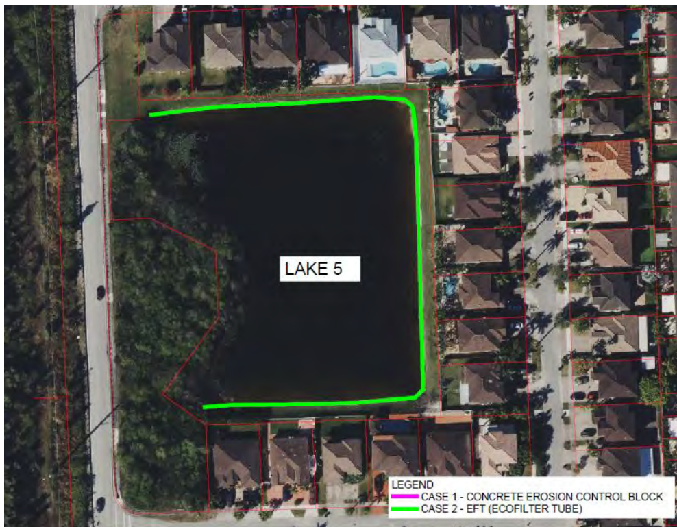
Figure 27: Aerial of recommended erosion control elements
