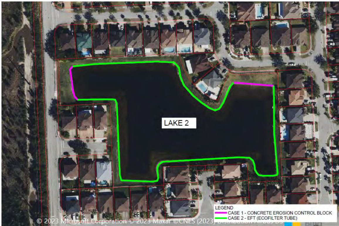
Figure 15: Aerial of recommended erosion control elements
