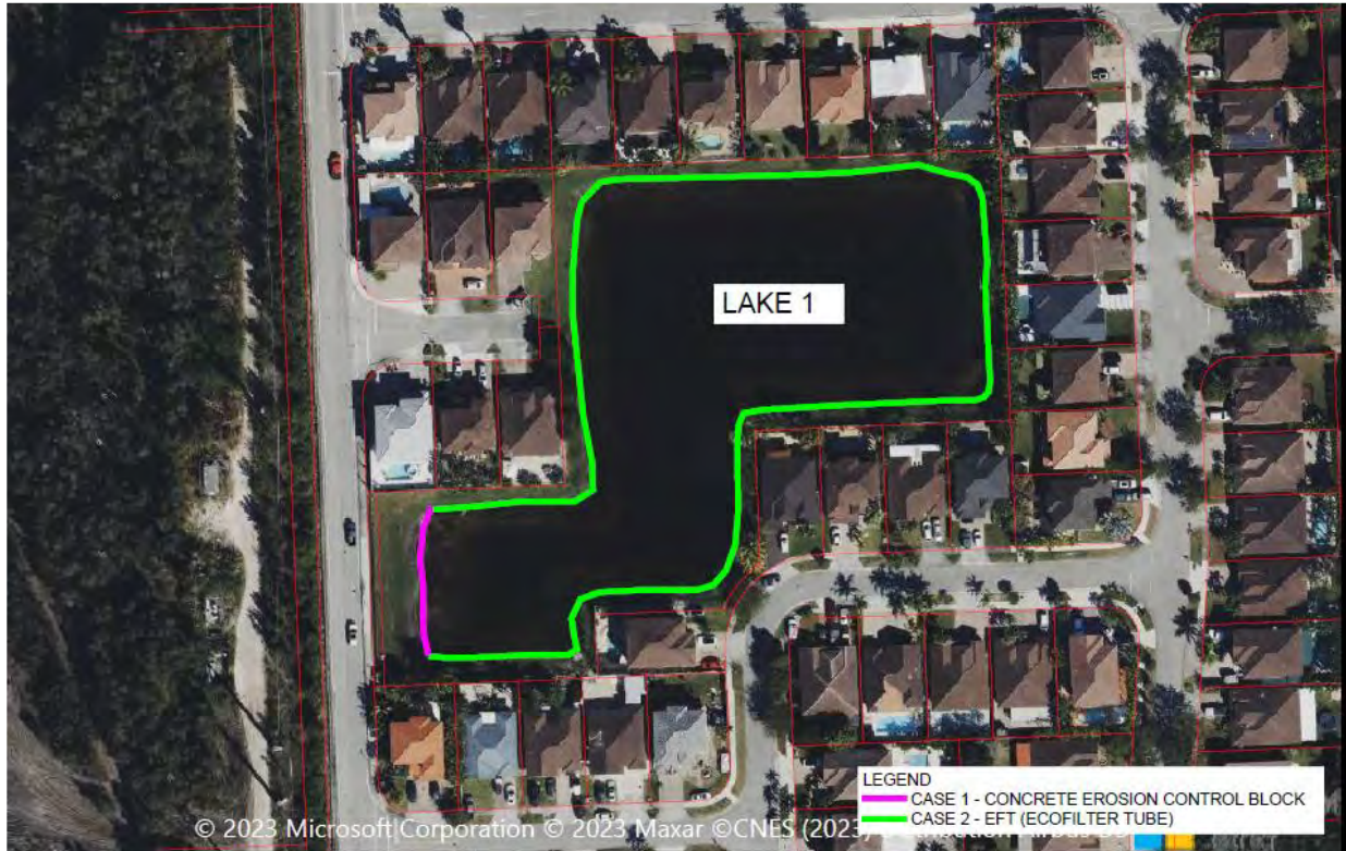
Figure 11: Aerial of recommended erosion control elements
