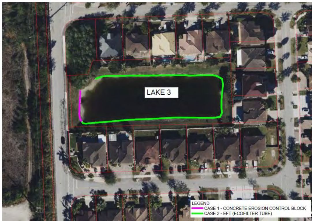
Figure 19: Aerial of recommended erosion control elements
